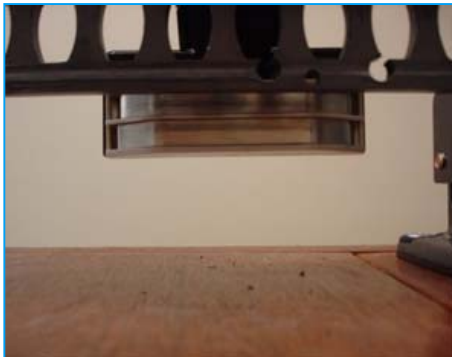
Figure 4-18: Contact de charge de rail
